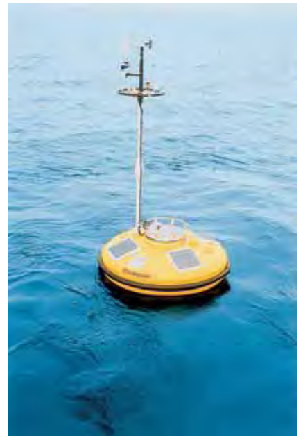
The PMB100 modules can be incorporated into data buoys to report barometric pressure at sea.
