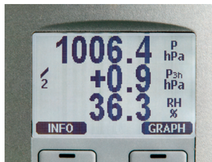
The display also shows the WMO pressure trend \Delta P 3h and tendency of 0 ... 9.
