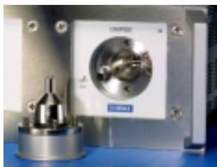
1. Remove the sensor cap.
