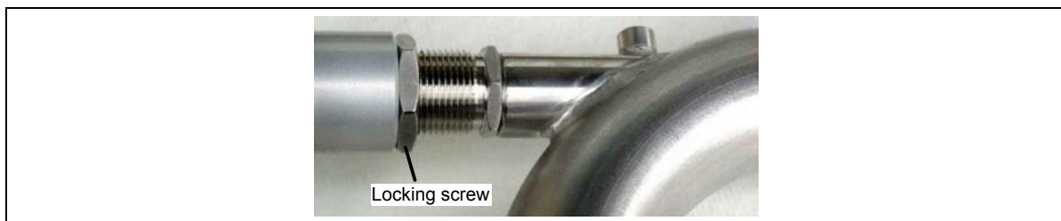
Figure 3.1. KS/2-P stroke length adjustment.
