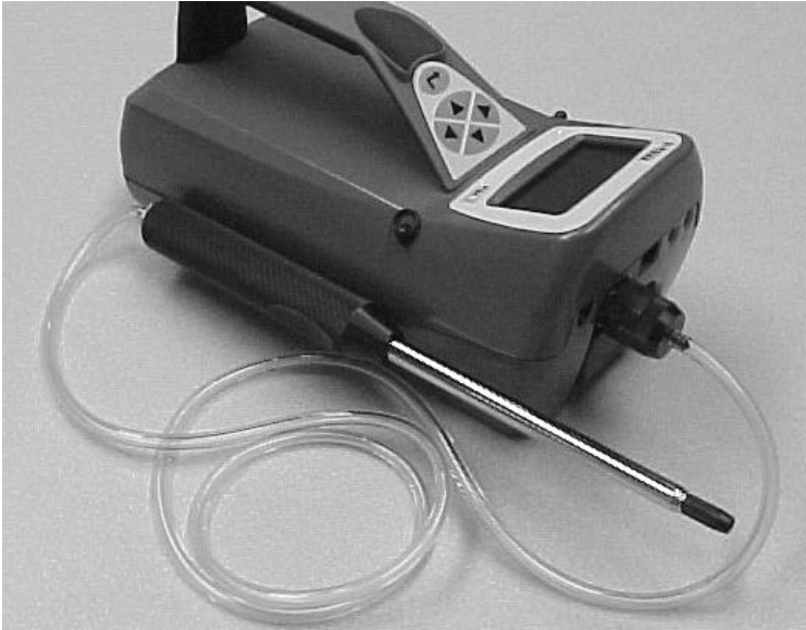
Figure 2-8: Slide Telescoping Probe Onto Instrument Case
