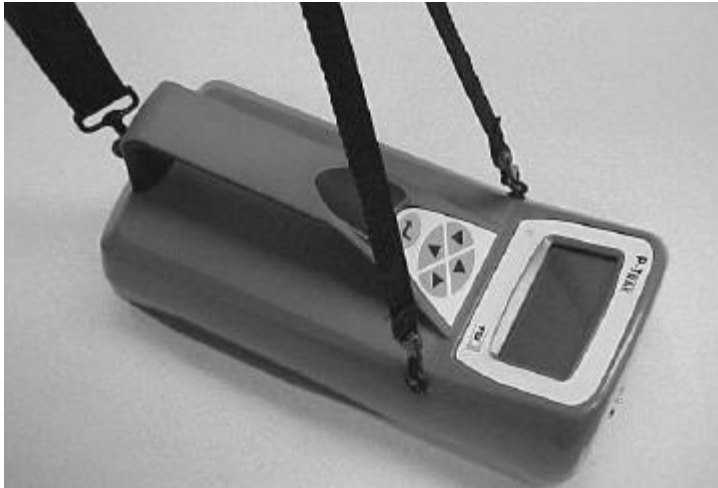
Figure 2-9: Attach Shoulder Strap to Instrument
