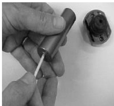
Figure 4-2: Remove Wick and Screen Using Dowel
