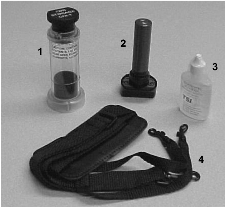
Figure 1-2: Alcohol Fill Capsule with Storage Cap, Alcohol Cartridge, Alcohol Bottles and Shoulder Strap
