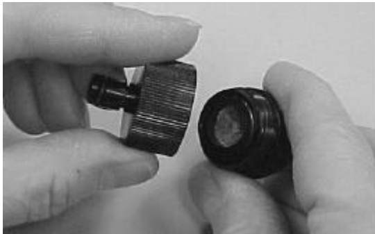
Figure 4-4: Re-assemble Inlet Screen Assembly
