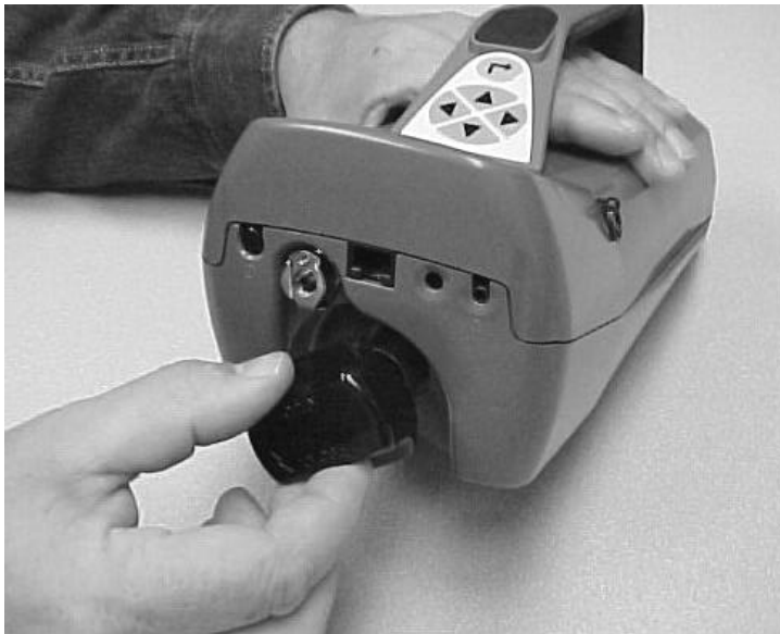
Figure 2-6: Insert Alcohol Cartridge into P-TRAK
