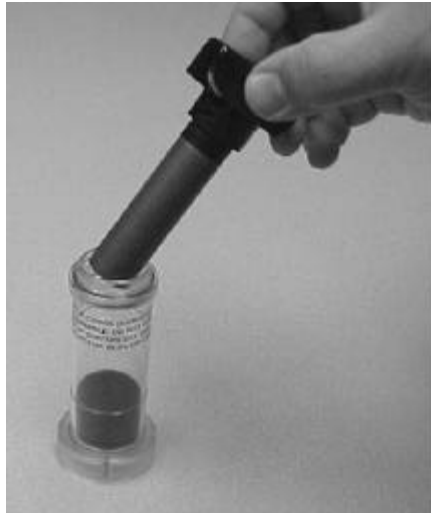
Figure 2-5: Insert Alcohol Cartridge into Fill Capsule
