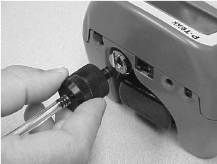
Figure 2-7: Insert Inlet Screen Assembly into Fitting
