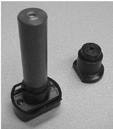
Figure 2-3: Alcohol Cartridge and Storage Cap
