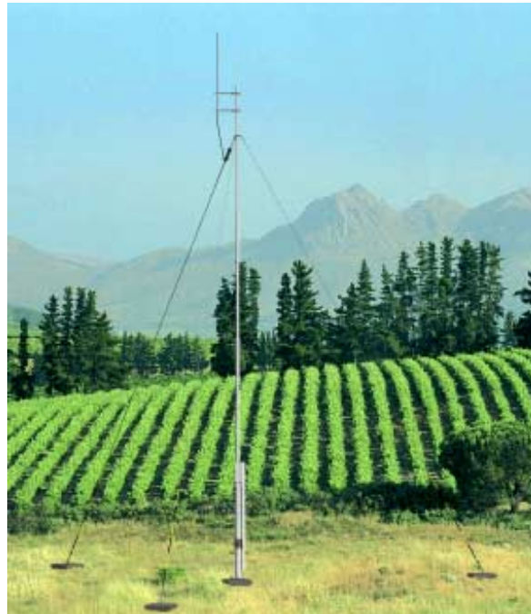
An Example of the 10-m Installation Mast with Accessories
