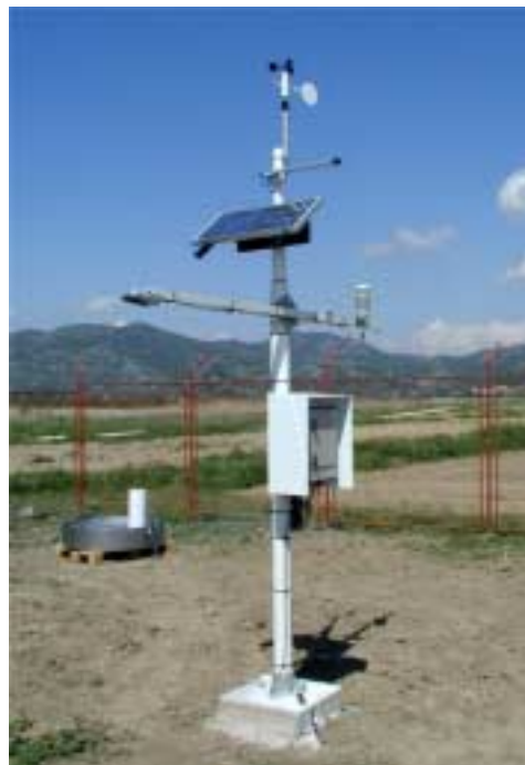
MAWS301 Automatic Weather Station Installation
