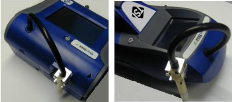
Figure 2-8: Installing Door-Oliver Cyclone
