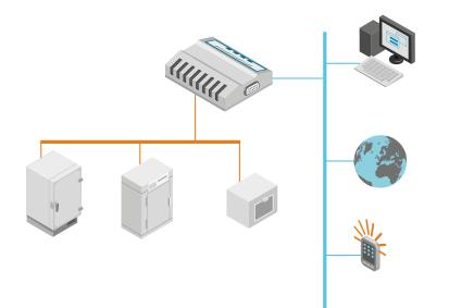
DL1016-1416 data loggers can be used with Vaisala software, either viewLinc or vLog, to download, display, and analyze environmental data.
