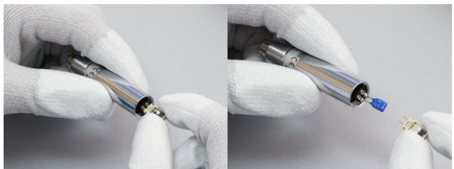
Figure 25 Removing the Sensor
