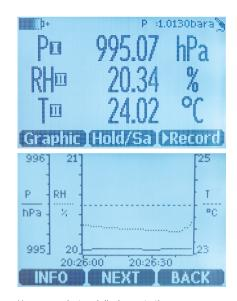
Users can select and display up to three measurement parameters at the same time. The graphic display shows the stabilization of measurement and process trends.
