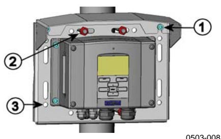
Figure 15 Mounting Rain Shield with Installation Kit
