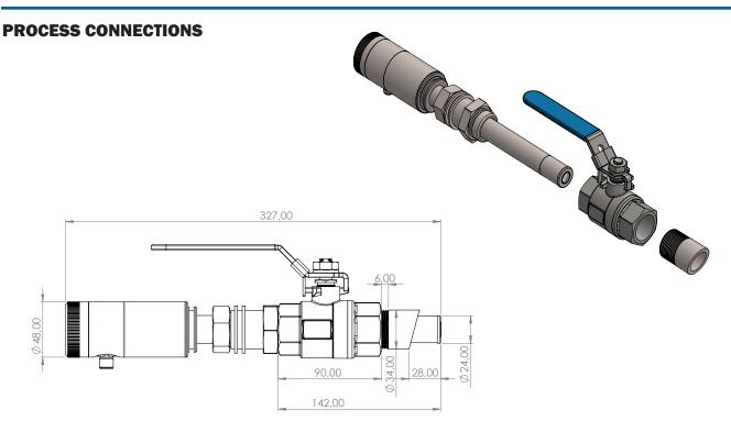
**Standard model:** VCA with process connection G1A ball valve insertion, G1 15° coupling, wetted parts material AISI316L, PG9 connection. Dimensions in millimeters. Selection code option B1. Coupling not included.
