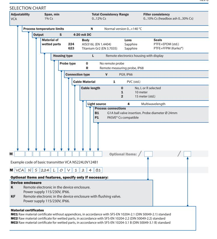
Example code of transmitter with remote electronics and material certificate VCA N S 224L0V124B1 K MC3
