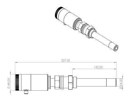
**Standard VCA sensor.** All dimensions in the datasheet are in millimeters (mm).
