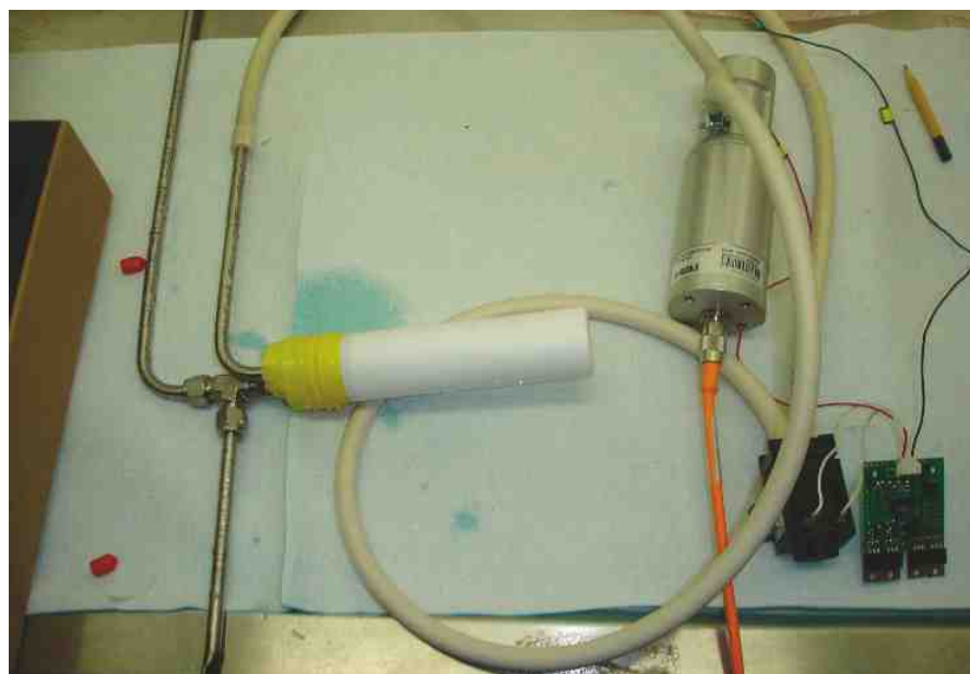
Figure 3. Test installation with a sintered PTFE chamber.
