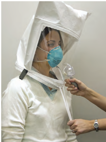
Qualitative fit test in progress.
