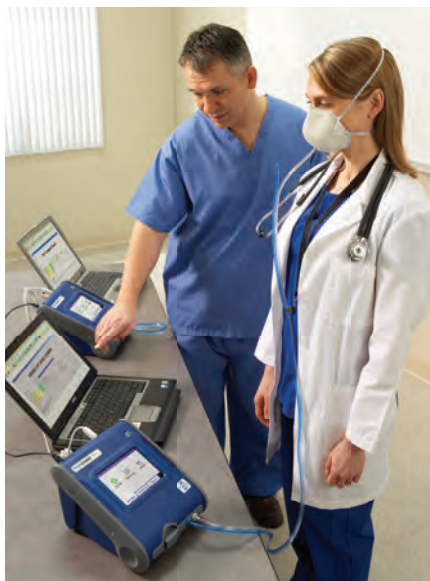
Quantitative respirator fit test in progress.
