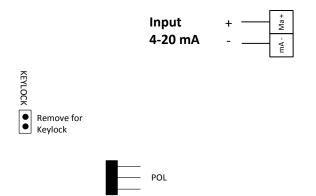
Connect the 4...20mA input to terminals 1 (+) and 2 (-). On models 301/302/305, refer to the polarity markings on the circuit board.
