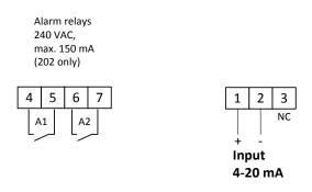
Models 301 and 302: connectors are located inside the device behind the display.
