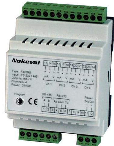
The transmitter 7470 provides an economical means of converting digital data to analog signals, mA / V, and transmitting them to four field instruments. Configuration is simple by MekuWin program or the general purpose hand held programmer 6790. The transmitter uses the simple Nokeval SCL protocol. One serial data bus accepts 31 7470 transmitters or other serial instruments, that is 124 output channels. Typical applications are PC-based programs or PLC.
