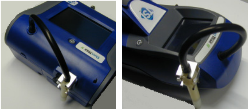
Figure 2-5: Installing Dorr-Oliver Cyclone
