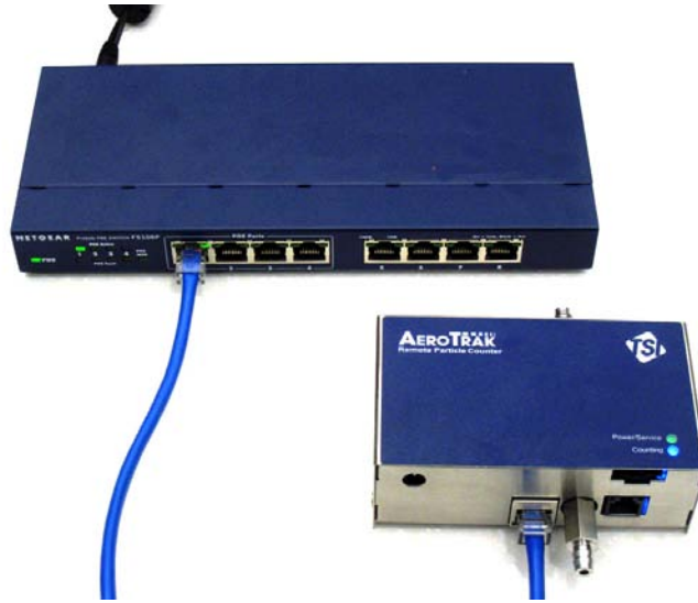
Remote Airborne Particle Counter Shown Powered by POE Hub
