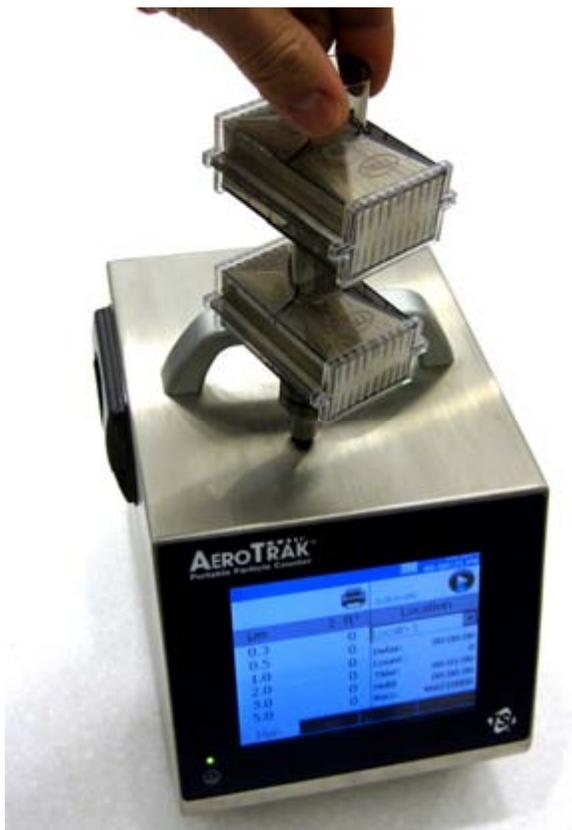
4. Press the
