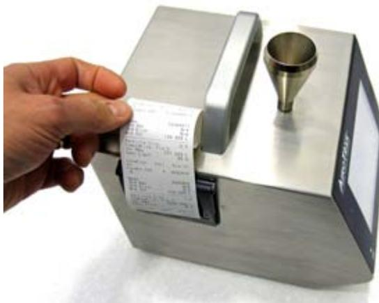
Printer paper has a colored strip printed on the last few feet of each roll to indicate time to change the paper roll.
