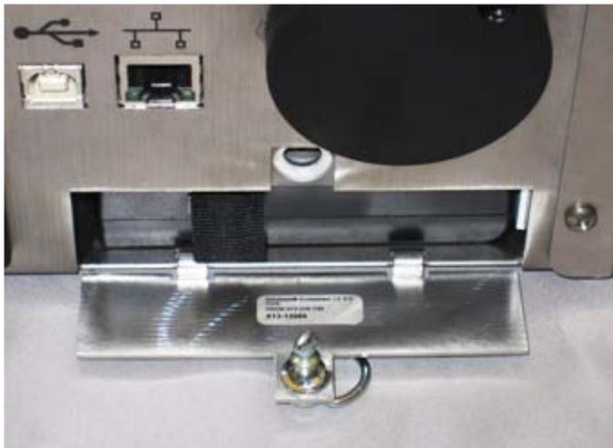
2. Slide the battery into the slot, pressing until it “clicks” into place (note that battery is approximately  $\frac{1}{4}$ -inch or 6-mm inside the back cover when properly installed.)
