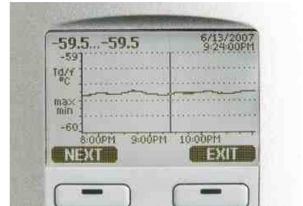
The display shows measurement trends, real-time data, and measurement history.
