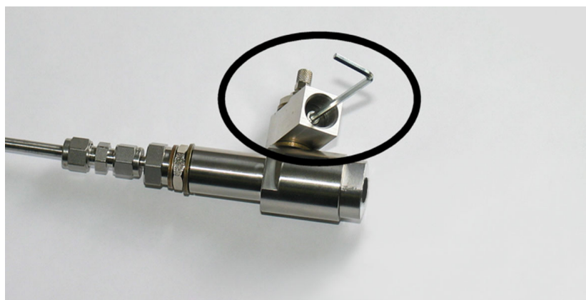
Figure 16 Removing the Leak Screw
