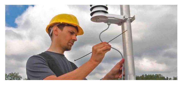
Outdoor humidity and temperature measurement is essential for applications such as energy management and indoor climate control. Just one outdoor humidity sensor typically optimizes the energy efficiency of cooling equipment. However, if this sensor is not accurate, both energy efficiency and human comfort may be compromised.
