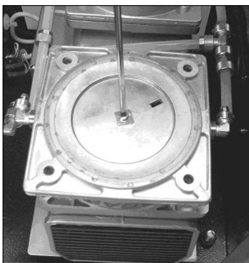
Figure 6.4. Replacing pump membranes, step 5.
