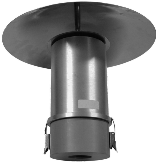
Figure 2.5. A PM10 sampling head.
