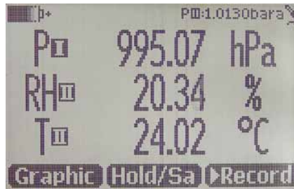
Some humidity measurement instruments allow an individual humidity parameter to be chosen which can then be followed on a graphical display. This picture shows different views of the Vaisala HUMICAP Hand-Held Humidity and Temperature Meter HM70 display.
