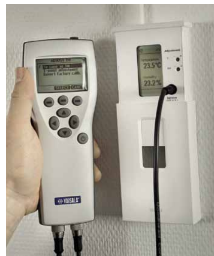
On-site calibration of a HMW90 humidity transmitter with a HM70 hand-held meter.
