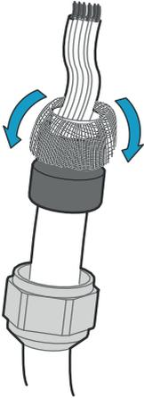
4. Lead the cable through the cable gland. Push the rubber seal back in place with the shield. Cut off any excess shield. Tighten the sealing nut with wrench (24 mm).
