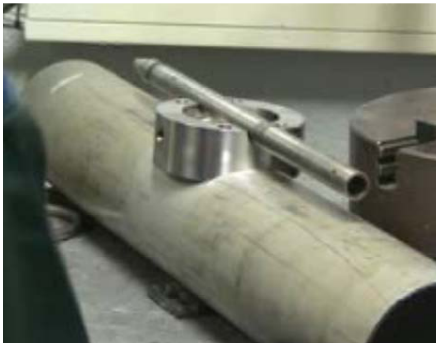
Figure 3-4 Installation of Pasve body C in horizontal pipe
