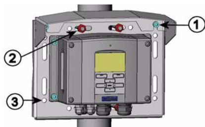
Figure 12 Mounting Rain Shield with Installation Kit
