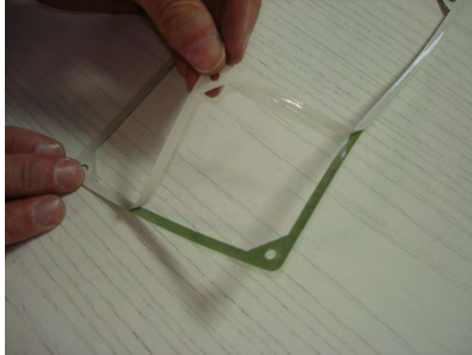
Fig. 7: Remove protective film from the sealing plate
