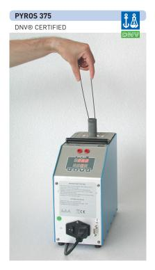
It covers a range from  $10 \,^{\circ}$ C above ambient temperature up to 375 °C. It has a stability of ±0,15 °C and an accuracy of ±0,25 °C at 150 °C. of ±0.35 °C at 375 °C.
