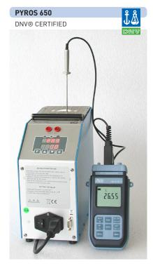
It covers a range from 15 °C above ambient temperature up to 650 °C. It has a stability of  $\pm 0,30$  °C and a all-range accuracy of  $\pm 0,50$  °C.
