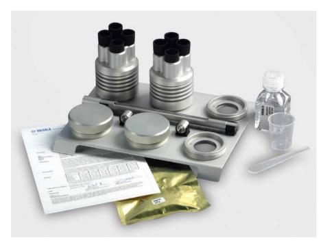
Vaisala Humidity Calibrator HMK15 for multi-point on-site calibrations.
