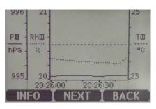
Some humidity measurement instruments allow an individual humidity parameter to be chosen which can then be followed on a graphical display. This picture shows different views of the Vaisala HUMICAP Hand-Held Humidity and Temperature Meter HM70 display.
