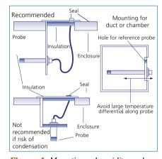
**Figure 1:** Mounting a humidity probe in a condensing environment.
