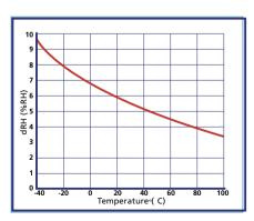
Figure 2: Measurement error at 100%RH at various temperatures when the temperature difference between the ambient air and the sensor is 1°C.
