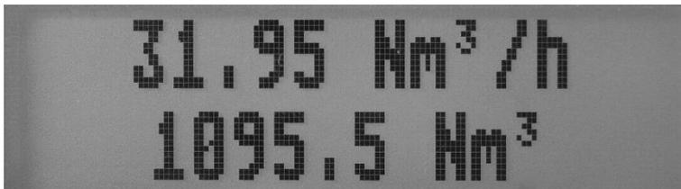
Row 1: current measured value – flow rate/mass flow/flow velocity
