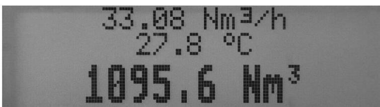
Row 1: current measured value – flow rate/mass flow/flow velocity
