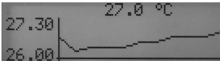
Here the current temperature is displayed in the heading and temperature values measured over the last 10 seconds are displayed graphically. The data runs from right to left with the oldest value on the left edge of the graphic.
