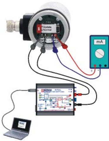
Wiring Housing with PLUG DIN43650- and M12-connector, test connector box, code HT & HS
