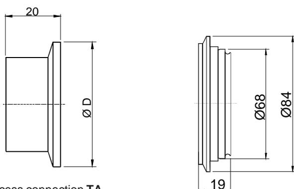
Process connection TA, TB and TC - Tri-clamp DN38 ... 63,5
