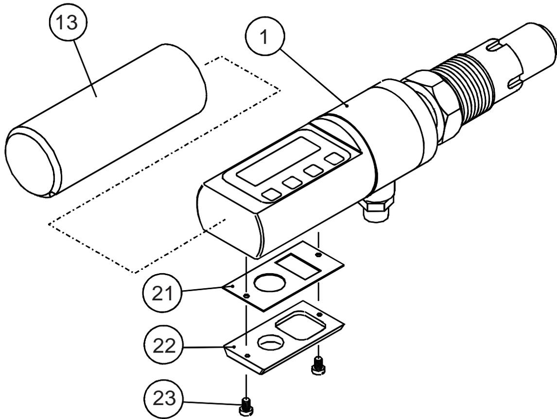
**Figure 5-1** Parts list: VDU with G1 thread with metal/metal taper process connection , sensor 1 (master)
