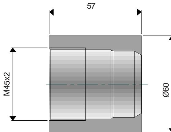
**SATRON VDU differential pressure transmitter with process connection M45x2 :**
