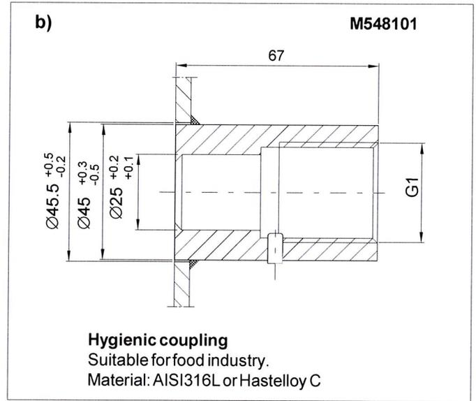
**Figure 1-10 Welded couplings**
