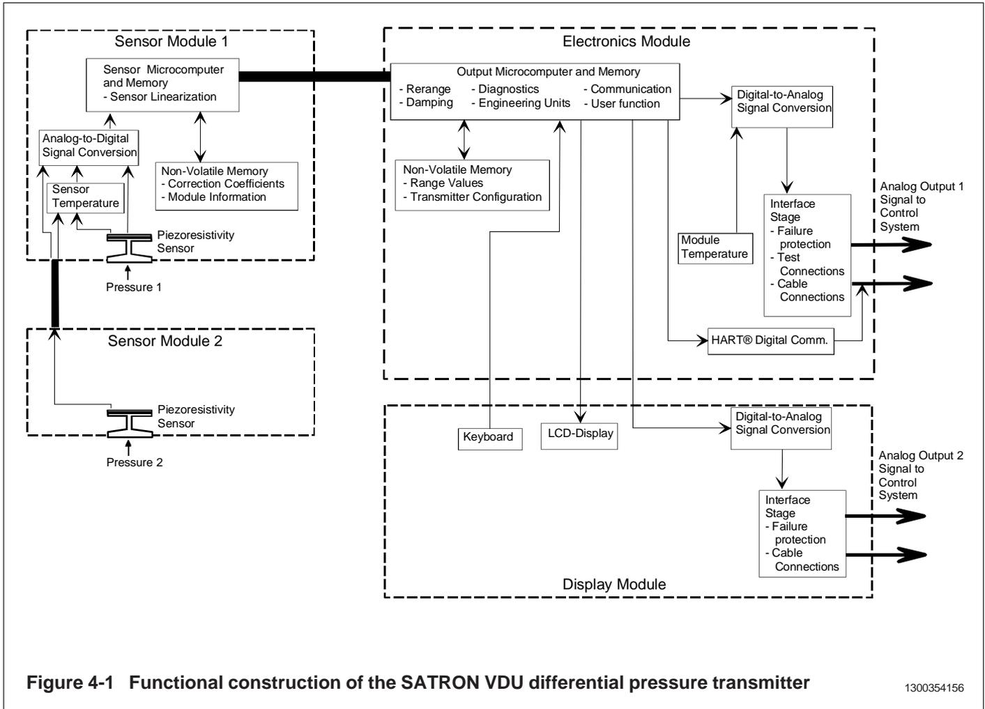
**Figure 4-1 Functional construction of the SATRON VDU differential pressure transmitter**
