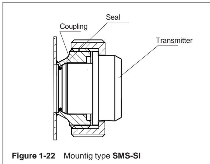
Figure 1-22 Mounting type SMS-SI
