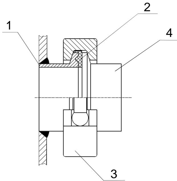
**Figure 1-20** Welded Tri-Clamp coupling
