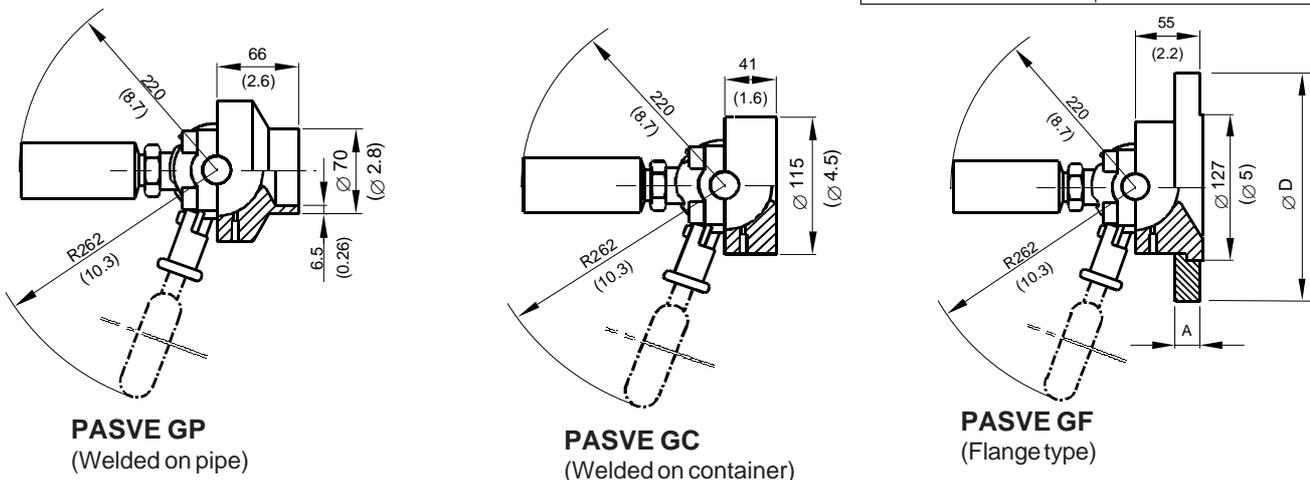
**Figure 1-16 Mounting dimensions for different PASVE® types**
