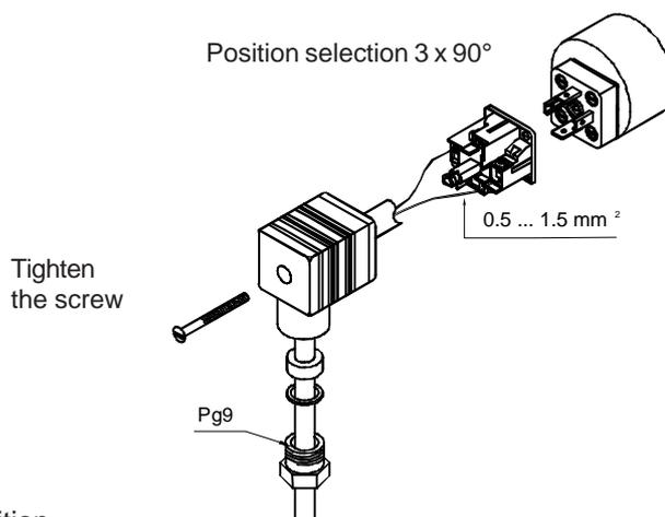
**Figure 1-25** Adjusting the junction box position
