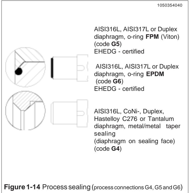
**Figure 1-14 Process sealing** (process connections G4, G5 and G6)
