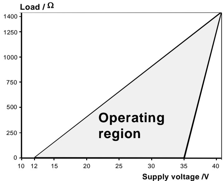
Min. load using HART® - communication 250 Ω
