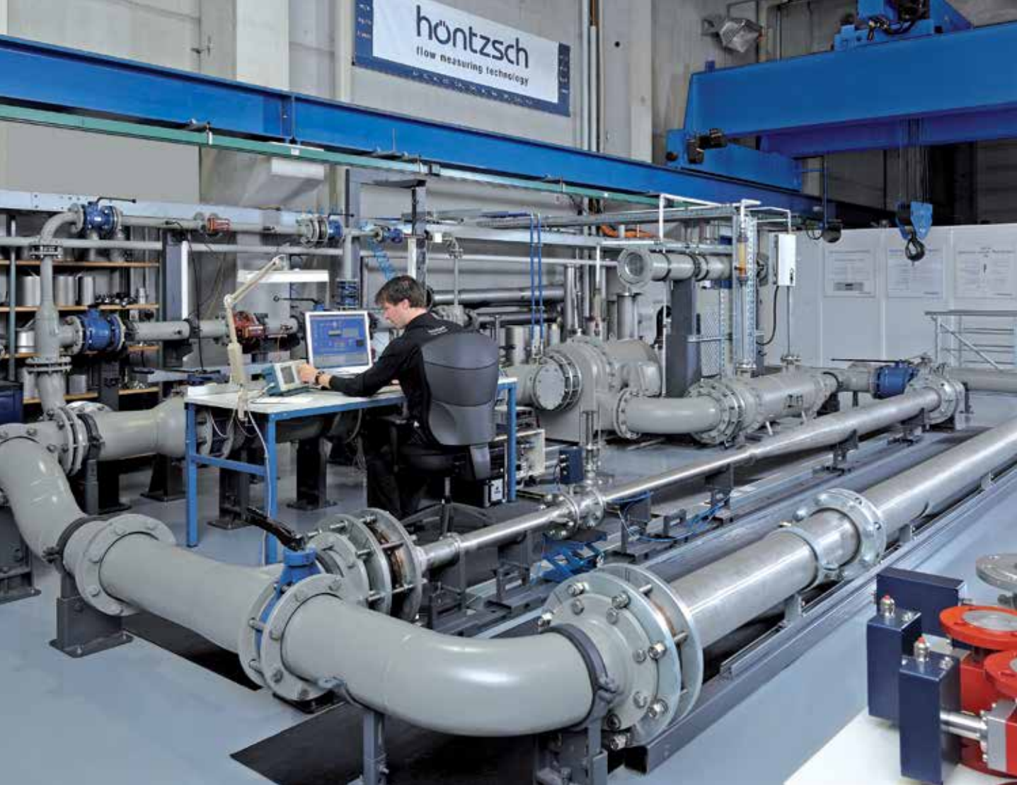
Volume flow calibration installation , range 0.20 ... 4000 m 3 /h, pressure up to 10 bar, 1 MPa, nominal value up to DN 200
