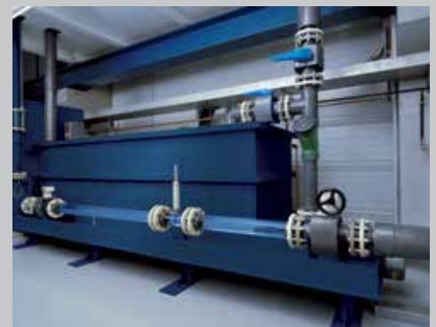
Water calibration installation , range 0.5 ... 120 m 3 /h, nominal values up to DN 150
