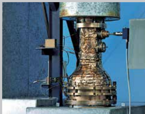
High temperature wind tunnel , +20 °C ... +400 °C, range 0.5 ... 70 m/s
