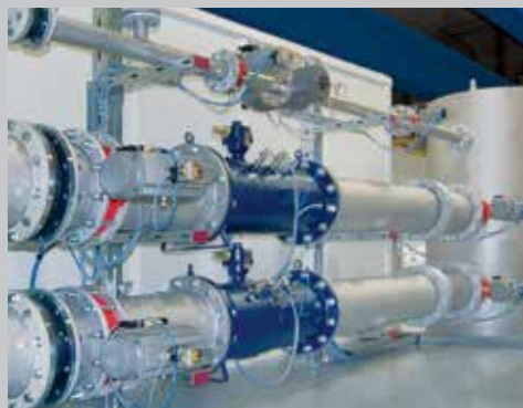
Atmospheric volume flow rate test facility , range 5 ... 5500 m 3 /h
