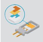
The HUMICAP sensor is a thin-film polymer capacitive sensor consisting of a substrate on which a thin polymer film is deposited between two conductive electrodes. The sensor surface is coated with a porous metal electrode to protect it from contamination and condensation. The dielectric properties of the polymer film depend on the amount of water absorbed. These properties change as the relative humidity around the sensor changes.
