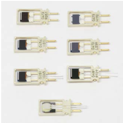
Family of HUMICAP sensors
