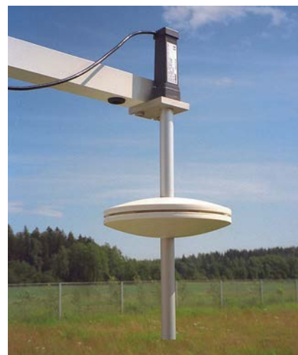
PTB210 paired with SPH10 static pressure head
