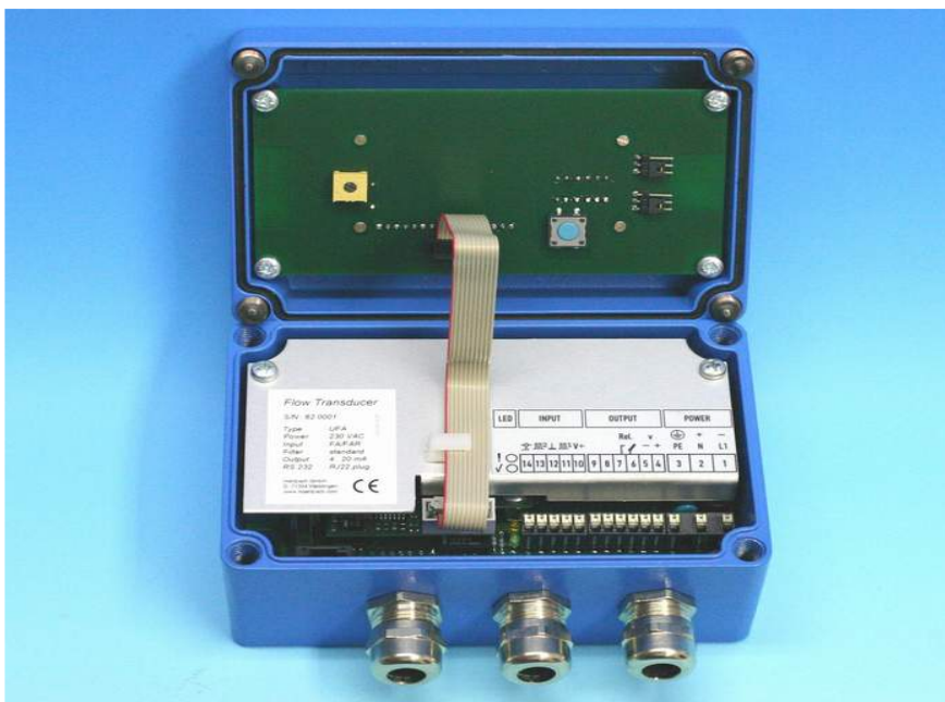
Fig. 2: LCD display connection with cover open
