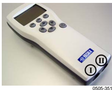
Figure 16 Location of the MI70 Probe and Cable Connector Ports
