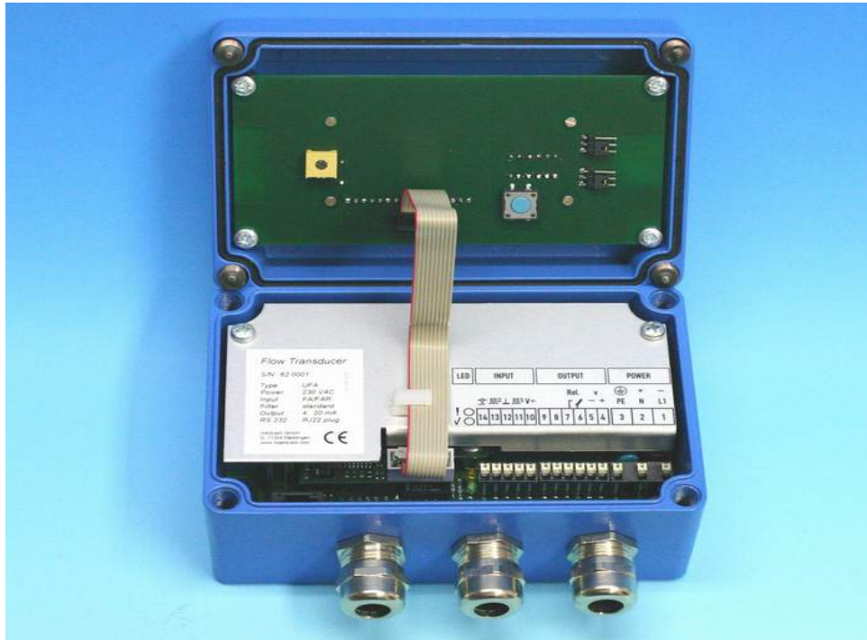
Abb. 2: LCD display connection with cover open
